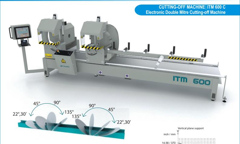
3-Axis controlled double mitre saw cutting-off machine, automatic traversing of the moving cutting head on slide ways and roller packs. Internal and external tilting of both heads. Any angle between 45° (internal) and 22°30′ (external) can be electronically set. Sawblade diam. 600 mm available with maximum cutting length of 4 and 5 meters.
